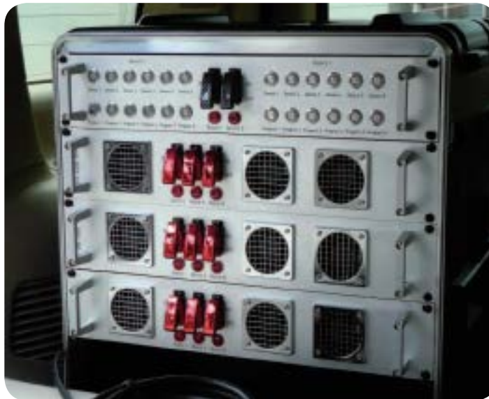
Jamming System with 1 Control Module and 3 Amplifier Modules (partial configuration)
