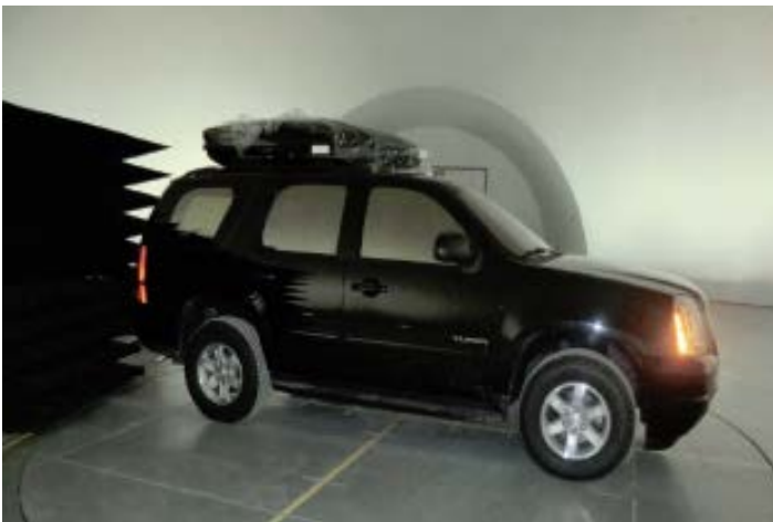
Measurement Radome - interior view Vehicle placed for RF shielding measurements on turning platform
