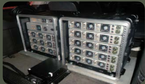
Jamming System with 1 Control Module and 3 Amplifier Modules (partial configuration)
